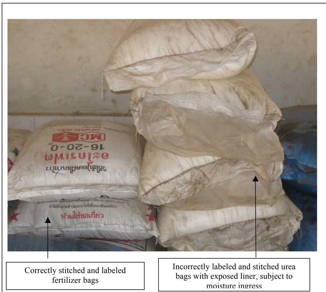
Figure 7: Picture of improperly stitched urea bags
