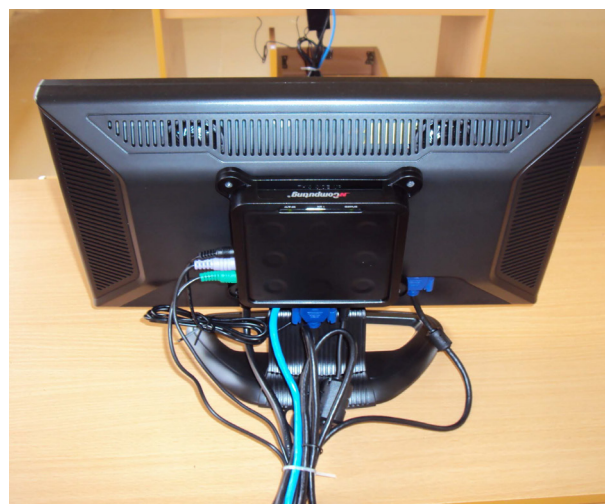
Revolutionary Technology: A Thin Client Device, so small it can be clipped to the back of a monitor.
