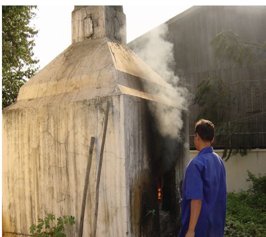
Medical waste incineration in Calmette Hospital
