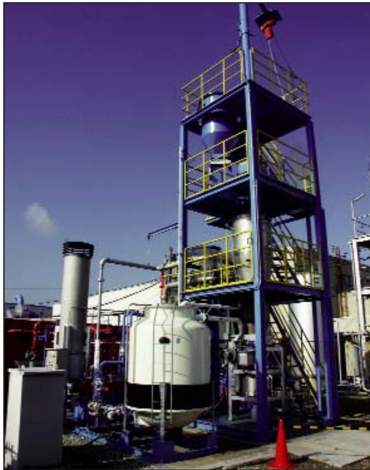
A Gasifier. Photo courtesy of Schmitt Enerotec GmbH.
