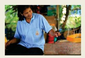
Throwing and Doubling: A worker (known as a throwster) twists the raw silk into different types of silk yarn by revolving by hand two or more strands of reeled silk using two sets of bobbins at different speeds to create stronger threads.
