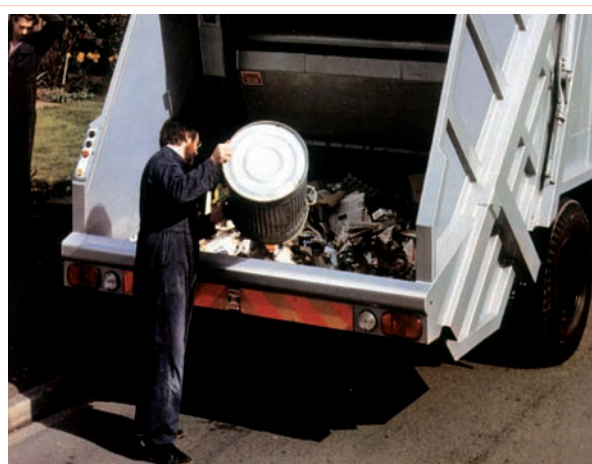
a) The low loading height and large hopper are big advantages
