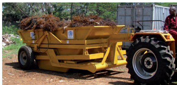
Figure 7.31 A very simple winch-on system can be used as a container lift or a conventional trailer
