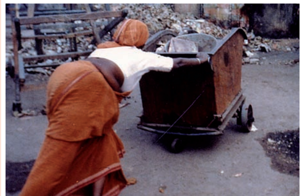
b) Badly designed cart (see also Section 7.3.1)
