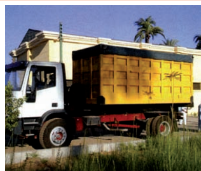
c) Container on specially designed tipping transport vehicle. Container capacity to suit waste density and truck load rating.
