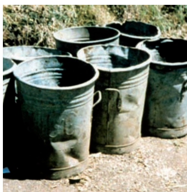
e) Thin gauge galvanised bins are easily damaged
