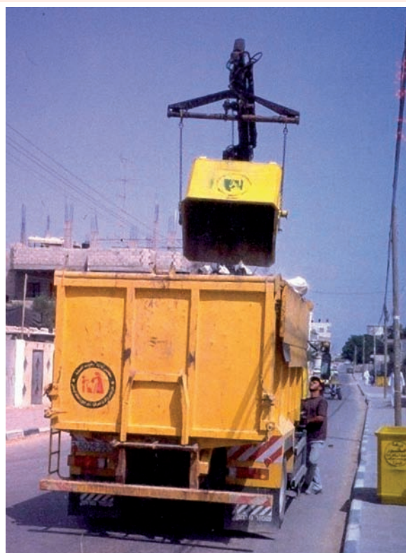
Photo 7.15 Crane tipper truck loading waste
