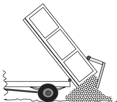
c) The tailgate is linked to the hinge by arms at either side and so is raised above the waste
