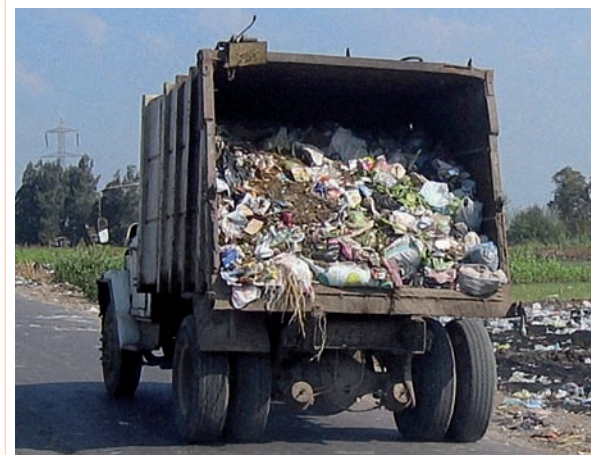
Photo 7.20 When the compaction mechanism cannot be repaired it can be taken off
