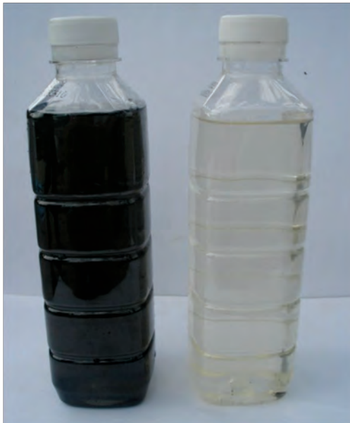
Picture 3: The color and transparency of wastewater before and after being naturally treated by the constructed wetland
