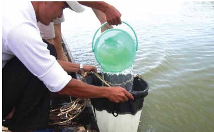
Step 2. Collect 10L of water and filter it slowly through the plankton net.
