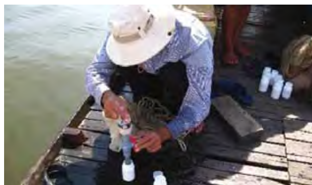
Step 5. Transfer the sample to a 250mL jar.
