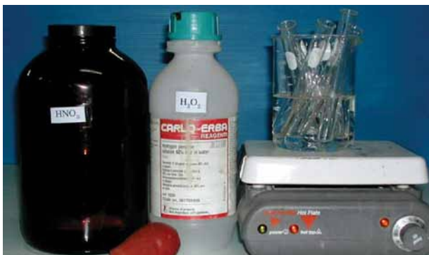
Step 3. Strong acid ( \text{H}_2\text{SO}_4 , \text{HCl} or \text{HNO}_3 ) is added and the tubes are heated ( 70 - 80^\circ\text{C} ) for 30 - 45 minutes.
