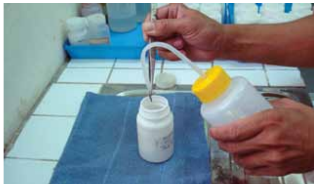
Step 1. Use forceps to remove large debris from sample.
