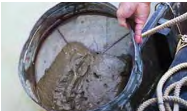
Step 4. Wash the sample, aquatic plants, and substrate, etc. by shaking the sample. Repeat many times.
