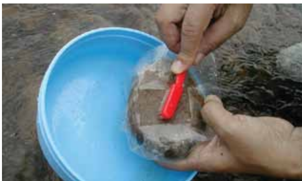
Step 5. Benthic diatoms on the surface of the selected stone are brushed off.
