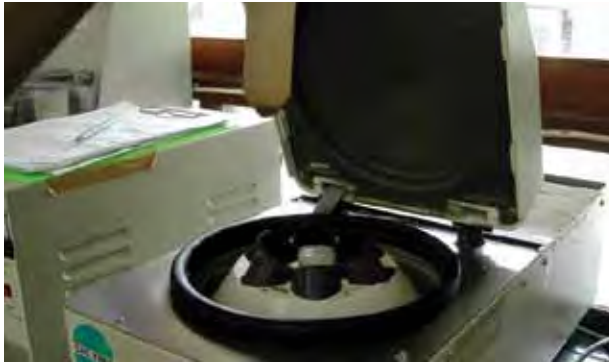
Step 1. The raw samples are centrifuged at 3,500rpm for 15 minutes.
