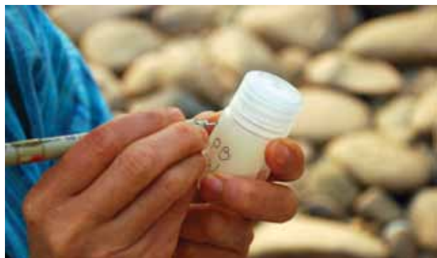
Step 7. The sample jar is labelled with the site name, site code, date, and sample replicate number.
