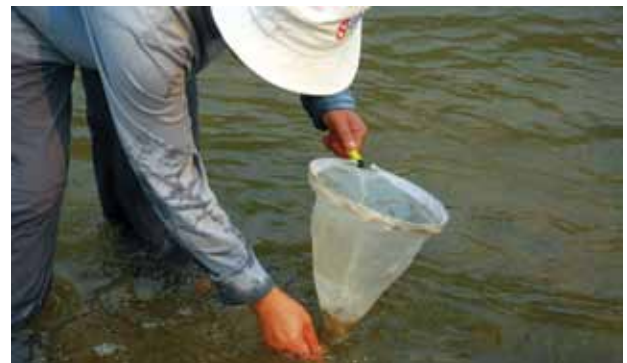
Step 3. The material adhering to the net is washed off with clean water.
