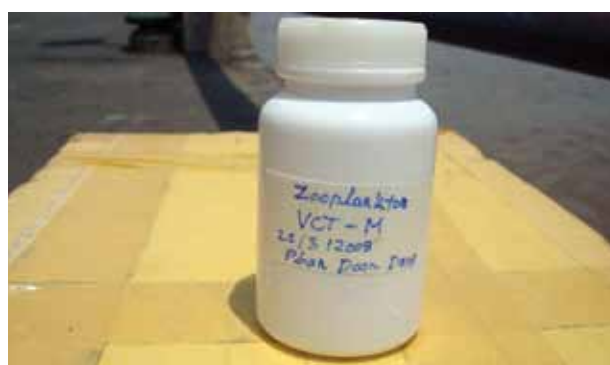
Step 7. Label the sample jar (site name, site code, date, location in the river).
